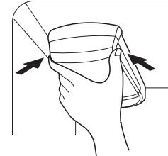
**3** Pull the water filter downward and turn it counterclockwise before pulling it out.
