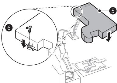
**2** Remove the screws from the rails at both ends.
