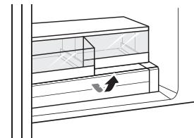
**3** Lift the front of the cover up with both hands until it detaches from the back wall of the cabinet, then pull it out.
