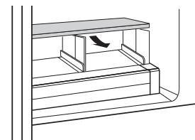
**4** To reassemble, insert the cover into the refrigerator with both hands and lower it onto the guides.
