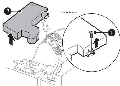
**2** Disconnect all wire harnesses **3**. Unscrew the ground wire **4**. Remove the cover.
