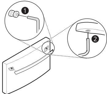
**1** Remove the screw **1** from the hinge cover at the top of the refrigerator. Lift the hook (not visible), located at the bottom of the front side of the cover **2** with a flat-head screwdriver.
