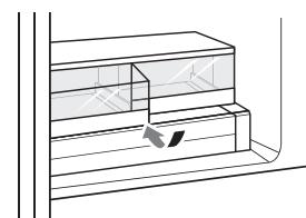
**6** Line up the tabs on the Door-in-Door case with the slots on the door and push down until it snaps into place.
