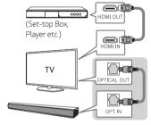
Set the input source by pressing OPTICAL on the remote control or pressing F repeatedly.
