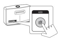
Initializing the network settings Press and hold **ADD** button until you hear the beep sound once. Then all wireless network ports are deactivated and delete the stored wireless network information.
