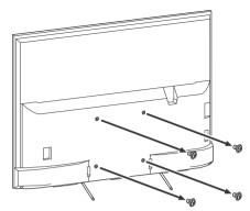
3 Attach the Attachment parts for Wall-Mount Bracket. Check the Attachment parts by referring to "1" of the Wall-Mount Bracket Installation Guide.
