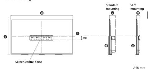
Screen **Display dimensions** centre Length for mounting dimension **Model Name** KDLa 0 G 0 e Standard Slim mounting mounting 65W850C 843 21 450 133 91 1,455
