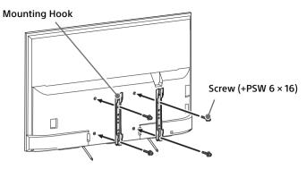
3 Make sure that the wall has enough space for the TV and is capable of supporting a weight of at least four times that of the TV. Refer to the following table on installing the TV to the wall. See page 20-22 (Specifications) for the TV's weight.
