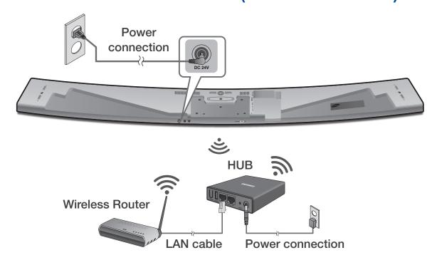
1 Connect a LAN cable to the router and the ETHERNET SWITCH on the back of the HUB.
