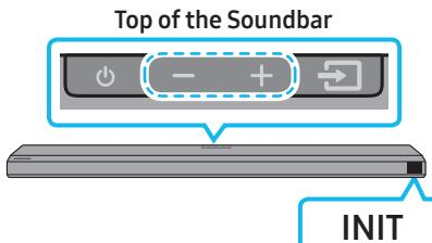
With the Soundbar on, press the **- + (Volume)** buttons on the body at the same time for at least 5 seconds. "INIT" appears on the display and then the Soundbar is initialized.
