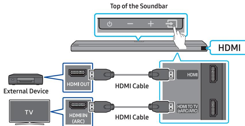
1. Use an HDMI cable to connect the HDMI OUT port on the external device and the **HDMI** port on the bottom of the Soundbar.
