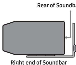
7. Install the Soundbar with the attached **Bracket-Wall Mounts** by hanging the **Bracket-Wall Mounts** on the **Holder-Screws** on the wall.
