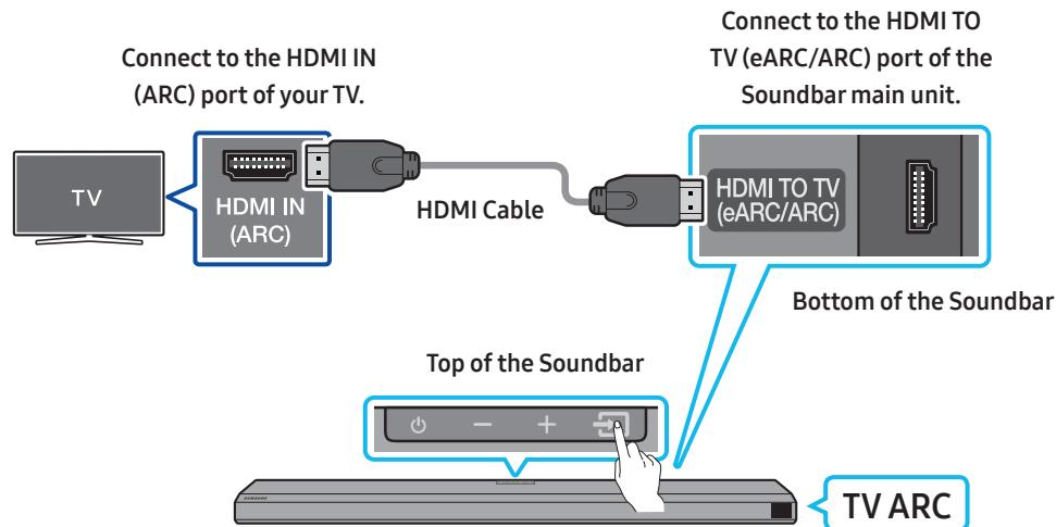
1. With the Soundbar and TV turned off, connect the HDMI cable as shown in the figure.
