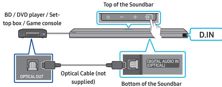
1. Use an optical cable (not supplied) to connect the **DIGITAL AUDIO IN (OPTICAL)** on the Soundbar main and the **OPTICAL OUT** port on the external device.
