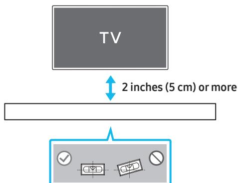
2. Align the **Wall Mount Guide's Center Line** with the center of your TV (if you are mounting the Soundbar below your TV), and then fix the **Wall Mount Guide** to the wall using tape.
