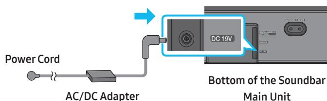
3. Connect power to the Soundbar and Subwoofer. The Subwoofer is automatically connected when the Soundbar is turned on.
