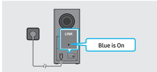
The LINK LED indicator stops blinking and glows a solid blue when a connection is established between the Soundbar and the Wireless Subwoofer.
