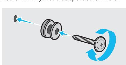
6. Install the **2 Bracket-Wall Mounts** in the correct orientation on the bottom of the Soundbar using **2 Screws**.
