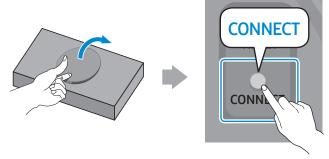
**2** Press the **CONNECT** button on the bottom of the Dial Controller.
