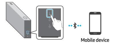
**2** Press and hold the **Multi-Function** button on Dial Controller until LED shows cyan. (for 2 seconds or more)
