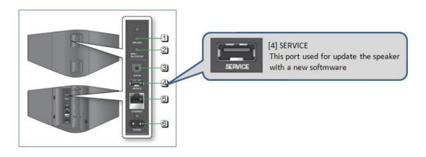
3. And then reboot the speaker. It will automatically download new S/W from USB. Or you can reboot the speaker by pressing Internet Radio Preset ( ) button.
