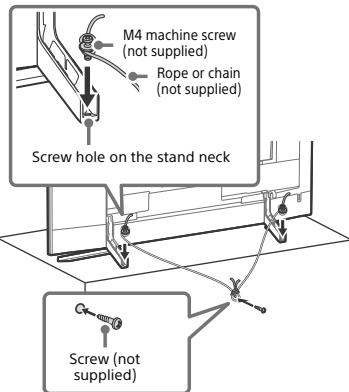
The length of the M4 machine screw differs depending on the rope or chain diameter. Please refer to below illustration.
