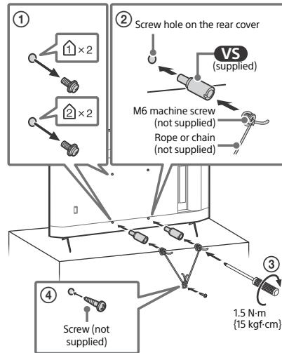
The length of the M6 machine screw differs depending on the rope or chain diameter. Please refer to below illustration.
