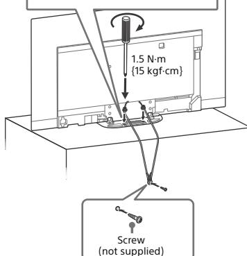
The length of the M4 machine screw differs depending on the rope or chain diameter. Please refer to below illustration.
