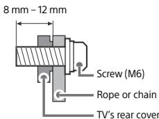
3 Anchor the TV to the wall by using bolts, wall anchor and chain (or rope).
