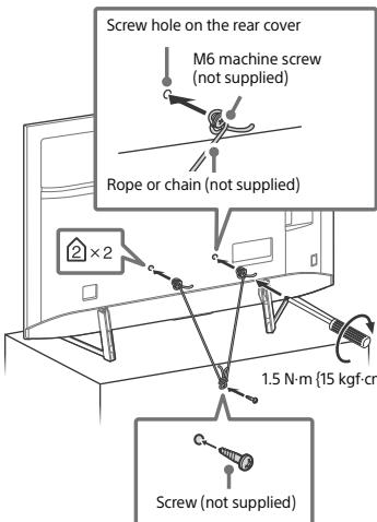
The length of the M6 machine screw differs depending on the rope or chain diameter. Please refer to below illustration.
