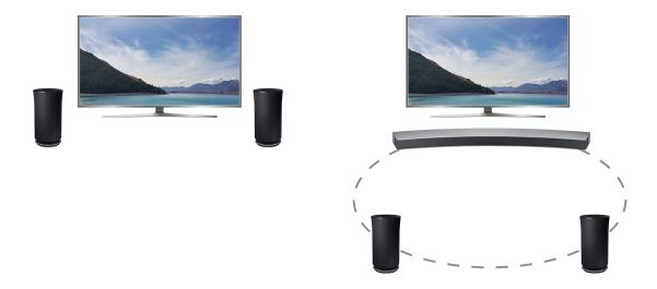
You can connect the TV to a Samsung wireless audio device through wireless network. At this time, two devices must be connected on the same network. For more information, refer to Wireless Speaker Manager ( > Settings > Sound > Expert Settings > Wireless Speaker Manager).
